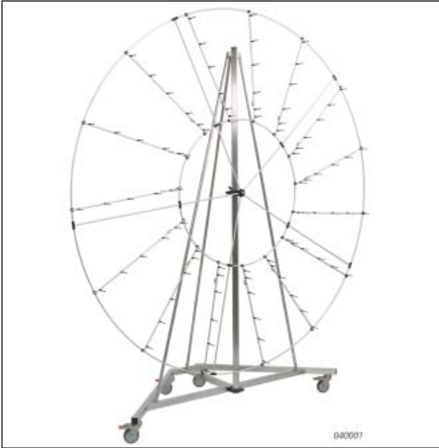
Fig. 16. Example of 90-channel wheel array with integrated cabling
